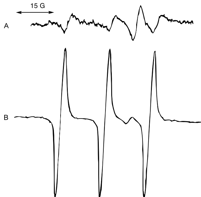
Fig. 3. ESR spectra from irradiation in PR-350 of tetramethylpiperidine (TMP), 1 , 7.7 mM, in methylene chloride for 15 min. (a) Without sensitizer, receiver gain (R.G.) of 5.0 \times 10^5 ; (b) with 9.2 \times 10^{-8} mol methylene blue, R.G. = 1.25 \times 10^5 , [R\cdot] = 0.14 mM. The peak on the high field part of the triplet, which appears here and in other spectra, is due to a permanent cavity signal.
